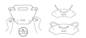
**Step 2A:** Assemble - Wearing gloves, locate P1 and P2. Insert each side of P2 into the inner most slots on P1. The arrow tabs on P1 should be facing away from you. Next, bend P2 to re-insert the arrow tabs, towards you, through the outter most slots on P1.
