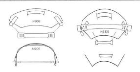
**Step 2B: Assemble -** Locate P3 and slide it over the arrow tabs from the inside of the shield. Use the slots to adjust how flat or concaved the shield is. Next, locate P4 and slide it into the slots on the bottom of the shield, from the inside.
